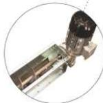
The bottom hopper has two vertical and two 60° sides. Running the length of the hopper is a sturdy 152mm trough auger with flights of different pitches to allow smooth discharge.
