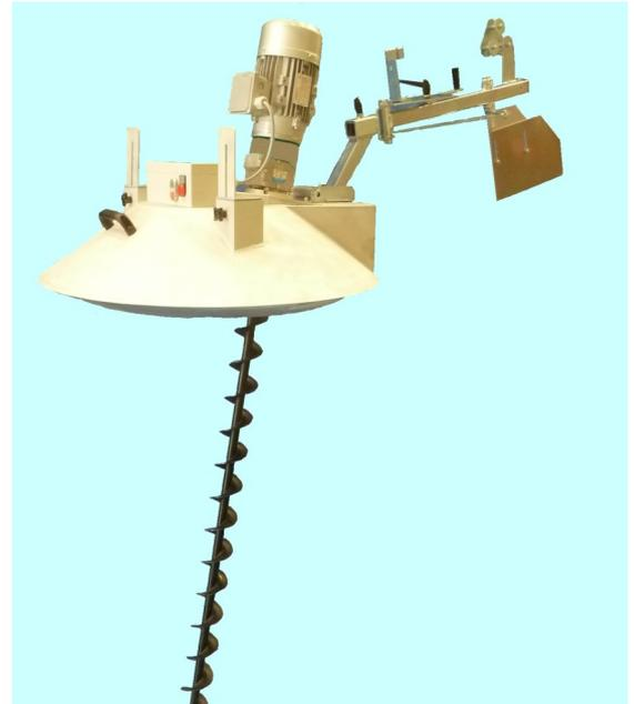
In addition, a rotary control system for a single Grain Butler can be fitted to allow the unit to "wind itself" towards a central point, thus minimising the need to turn the unit.
